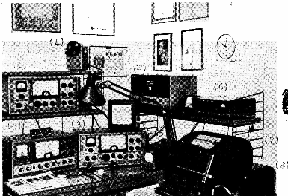
The RTTY station of IILCF, operated by Dr. Franco Fanti, Via Alberto Dallolio 19, Bologna, Italy, who runs Geloso transmitters (types 220 and 225), the T/P machine being a TG7B Teletype with auto-transmitter head. His main receiver is a Geloso R.209. He also has an automatic "CQ-caller" for RTTY.
